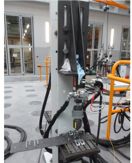
Hilti S-BT fastening system under cyclic loading
