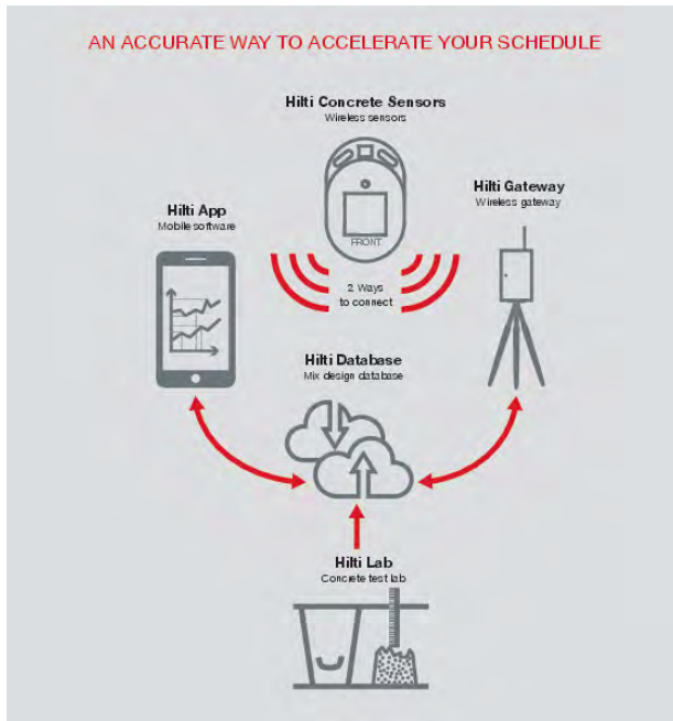
Fig. 9.21: Hilti concrete sensor system solution
