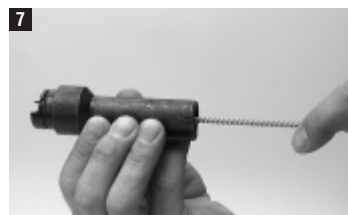
7 Inside of fastener guide
